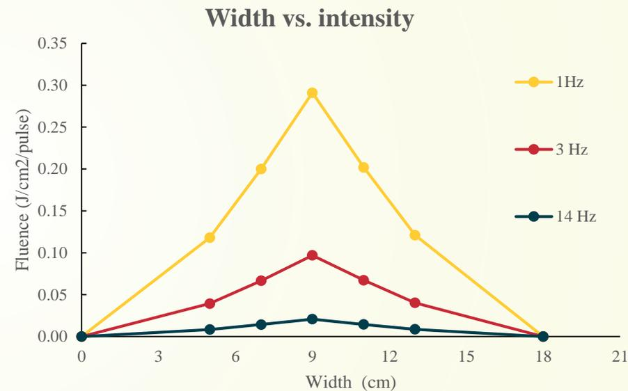
**The uniformity of IPL energy distribution, especially the length direction is improved significantly over the earlier IPL system**
