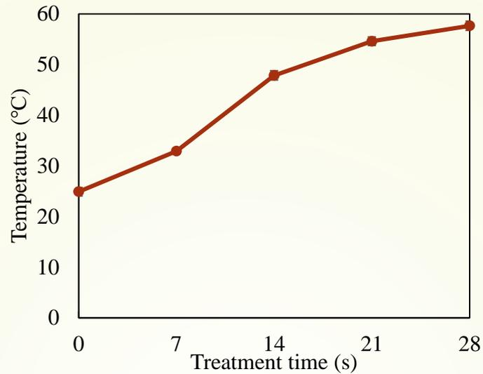
Temperature profiles of NFDM treated in the **original IPL system** after 28
