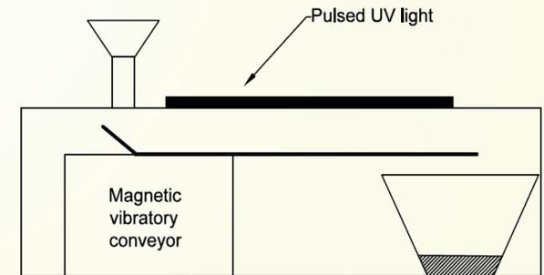
**Vertical fluidized bed and horizontal shaker/vibratory designs**
