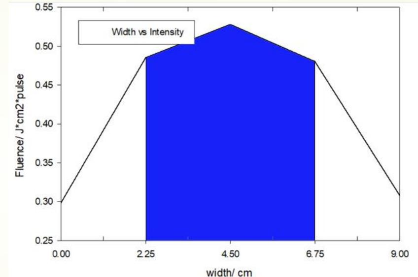
The IPL energy (J/cm<sup>2</sup>/pulse) distribution on the vibrator surface. The highest influence area below the IPL lamp is marked in diagram with blue color.
