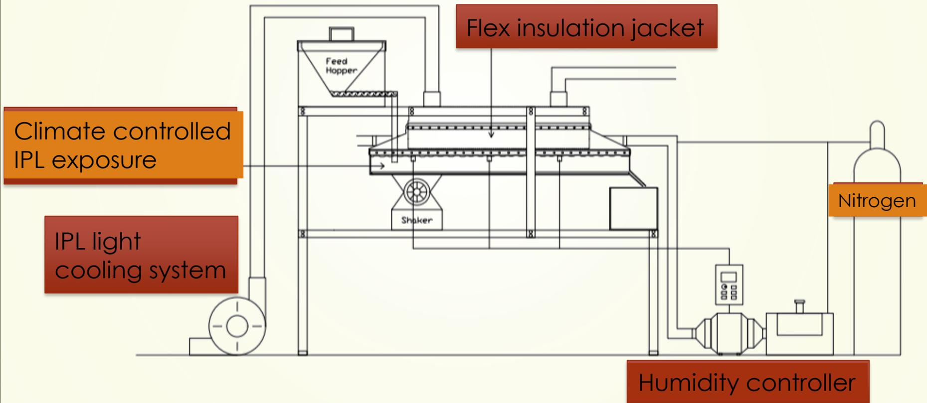
Subsurface cooling was added to extend substrate retention time
