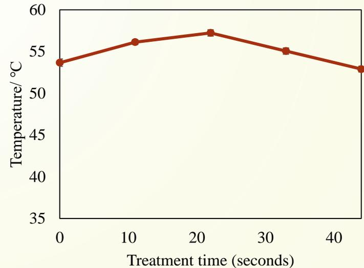
Temperature profiles of NFDM treated in the **improved IPL system** for 28 and 44 s, respectively.
