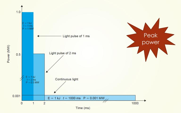
Power delivered by continuous light and light pulses of different duration, having equal energy content.
