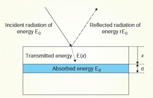
The absorbed light energy is generally dissipated as heat, resulting in a temperature increase equal to:
