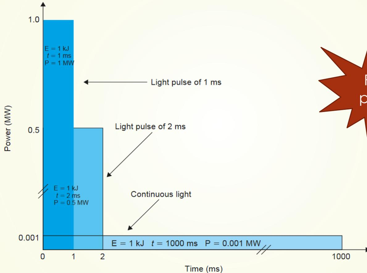
Power delivered by continuous light and light pulses of different duration, having equal energy content.
