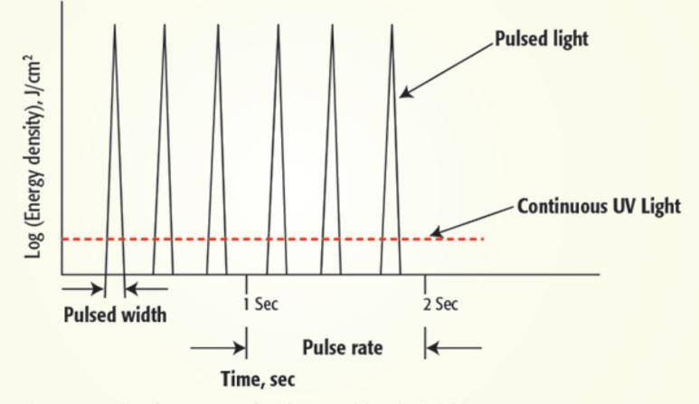
Figure 4: Comparison of Energy Output of Continuous UV Light and Pulsed Light
